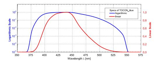
GaP blue light detector with integrated amplifier
